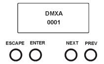
After switching the fixture on, display shows current DMX address.
